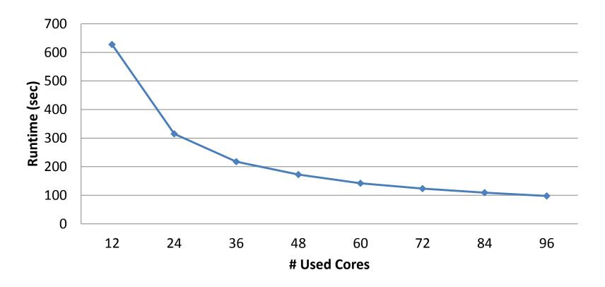
Factorization of 100 predefined input numbers Client Intel 2 Core, 2.9 GHz; Service Intel 2 Core, 2.9 GHz; 64 Bit, with Compiler Optimization Cluster MS HPC 2012, 32 Nodes Intel Xeon 12 Core 2.6GHz; 100MBit/s network, 1ms delay
