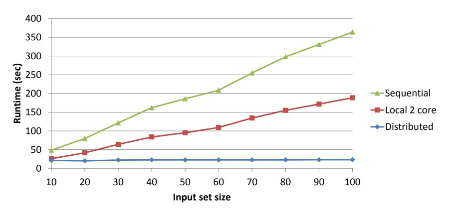
Factorize a set of predefined numbers; Minimum of 3 measurements; Client Intel 2 Core, 2.9 GHz; Service Intel 2 Core, 2.9 GHz; 64 Bit, with Compiler Optimization Cluster MS HPC 2012, 32 Nodes Intel Xeon 12 Core 2.6GHz; 100MBit/s network, 1ms delay
